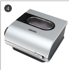
Close the flip lid, ensuring that it clicks into place.
